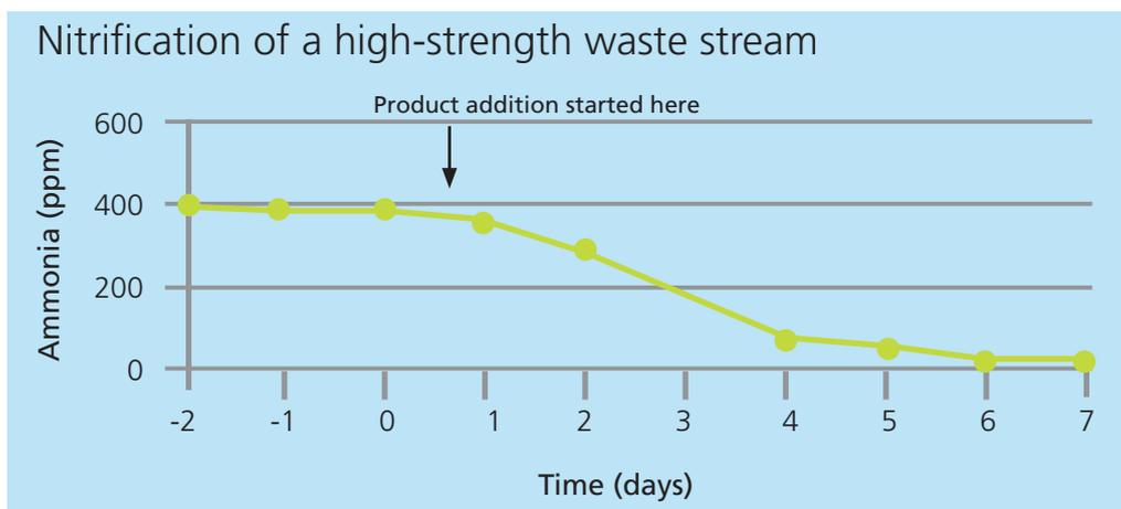
Fig. 2. Recovery of nitrification at a chemical plant.
