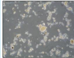
Pin floc (left) can lead to excess solids loss from the clarifier and contribute to nitrification problems.
