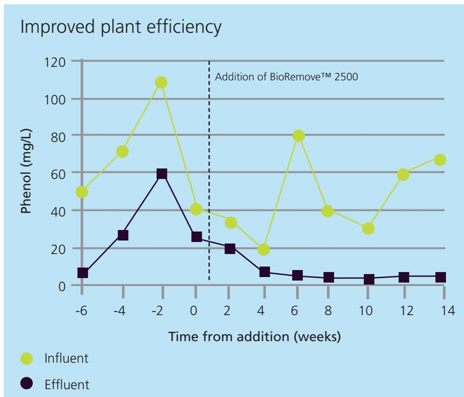
Fig. 1. This chart demonstrates phenol reduction as a result of the addition of Novozymes BioRemove™ 2500. The effluent phenol significantly drops over time enhancing the plant stability in a refinery wastewater treatment system.
