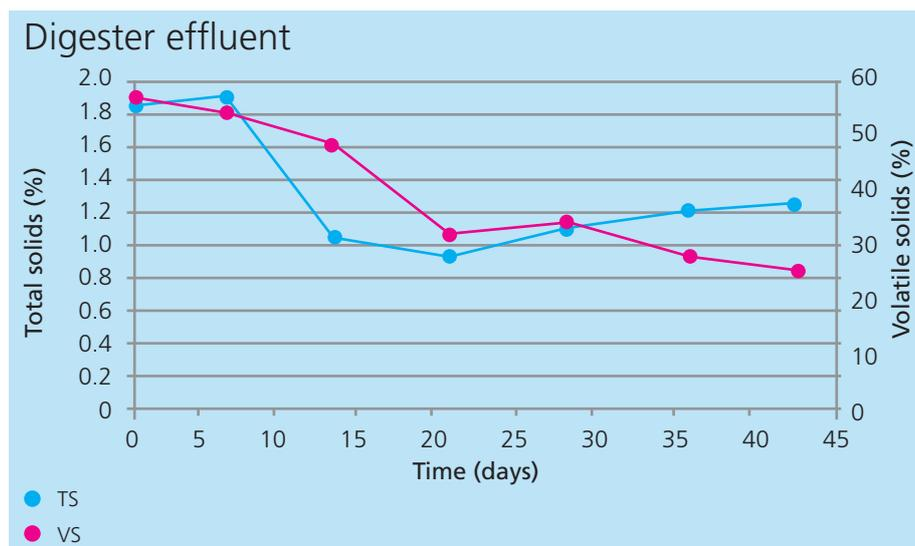
**Fig. 2.** The reduction in solids allowed the digester to be fully operable in less than 60 days without any additional costs due to physical solids removal, saving the facility nearly USD 750,000.
