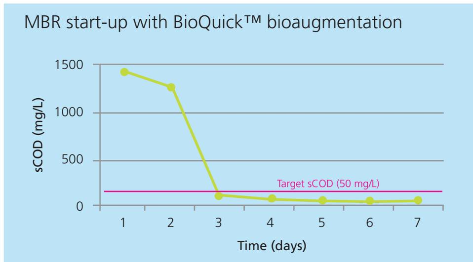
Fig. 2. COD reduction using Novozymes BioQuick 5130.
